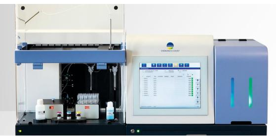
The fluorescence ratio is used to differentiate labeled microorganisms from other particles from the food item. Final results are reported following digital data processing.
